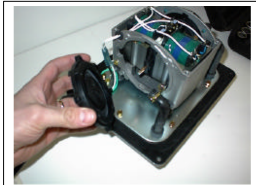
J. Remove diaphragm holder (11).
