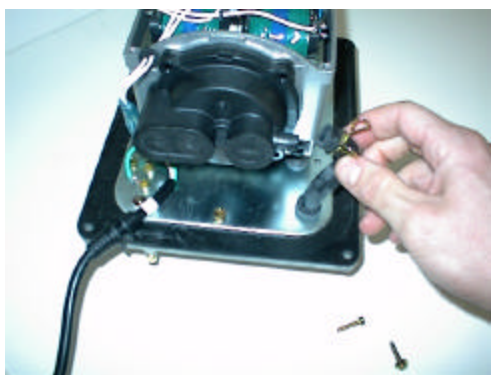
G. Disconnect connecting Pipe (13)
